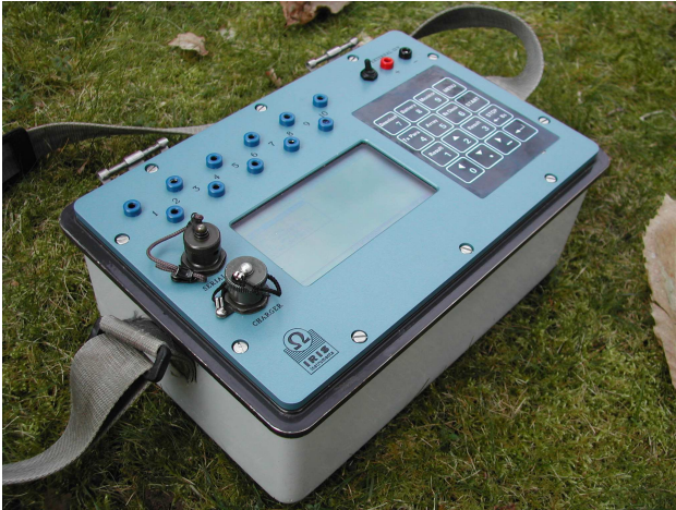
ELREC Pro unit with its graphic LCD screen
